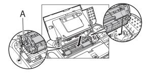
Push the toner cartridge to make sure it is properly set in the machine.
